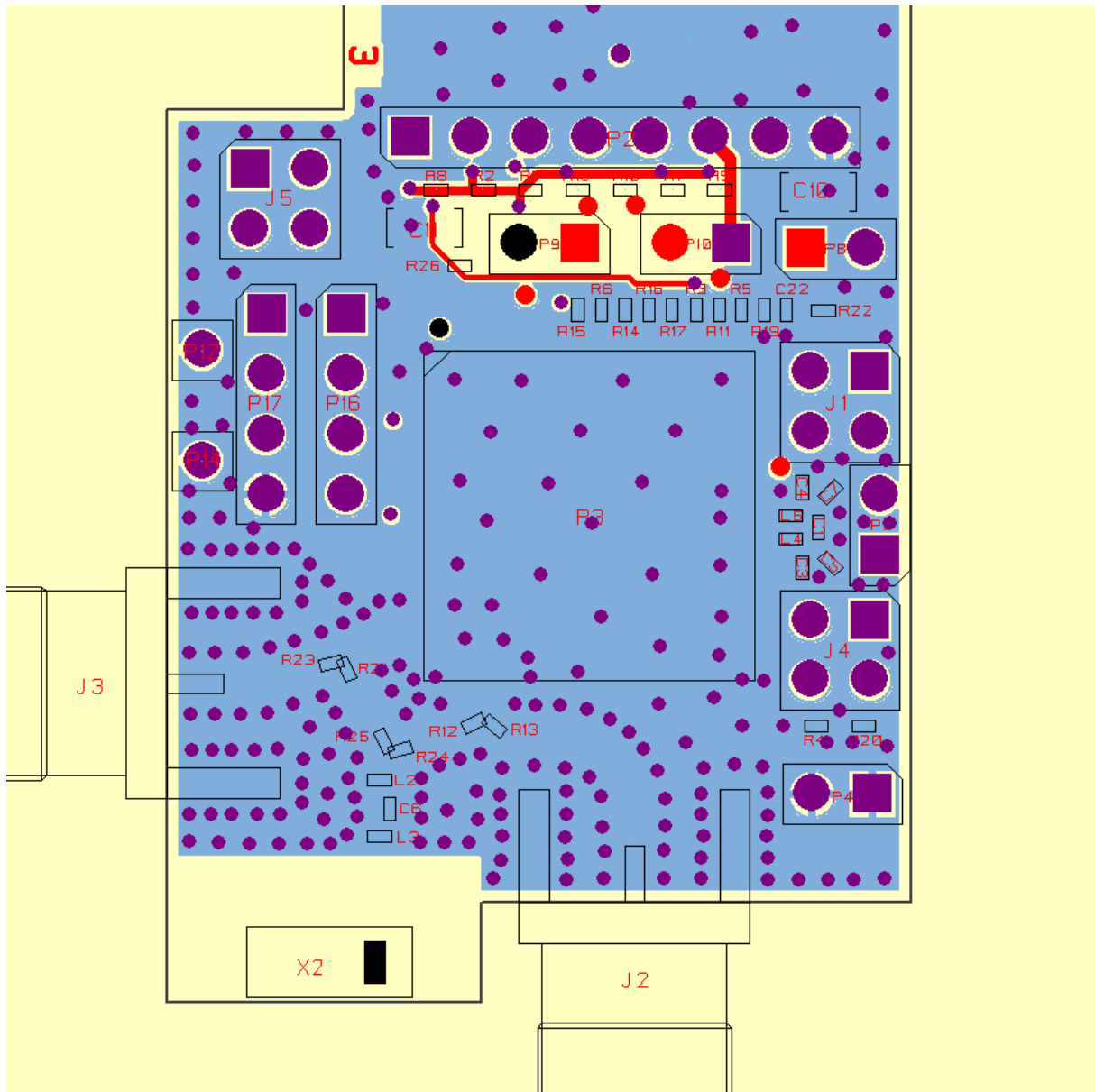
Figure 6. Third layer, ground and supply.
