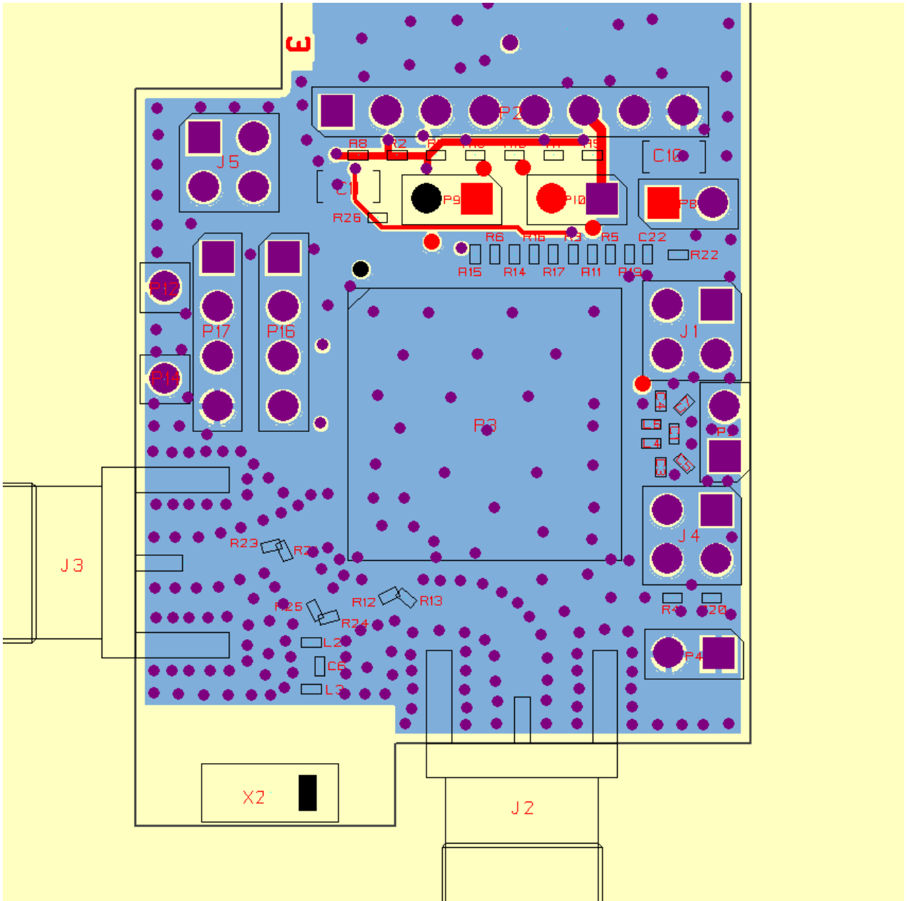
Figure 6. Third layer, ground and supply.
