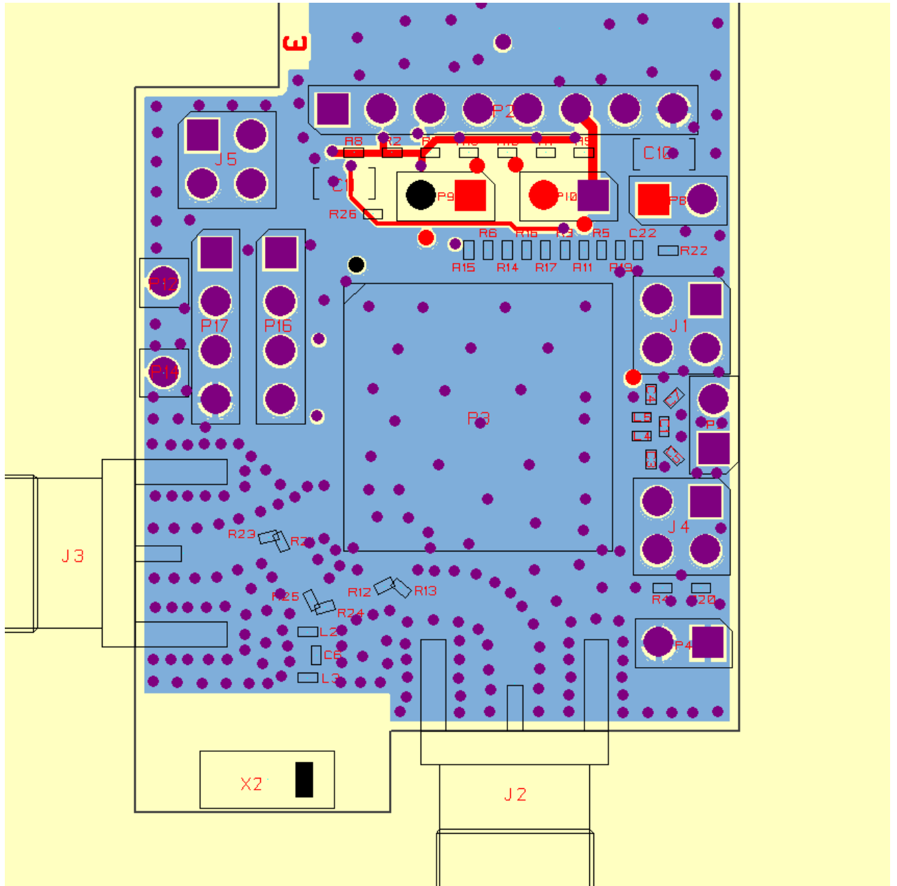
Figure 6. Third layer, ground and supply.
