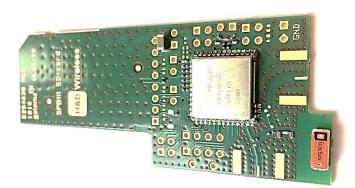
• The SPB209A EVB (SPB209A mounted on the SPB111 SD carrier card). Using the onboard dual antenna.
